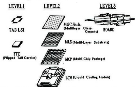
Fig.1 Packaging hierarchy for NEC ACOS 3800 computer system.
